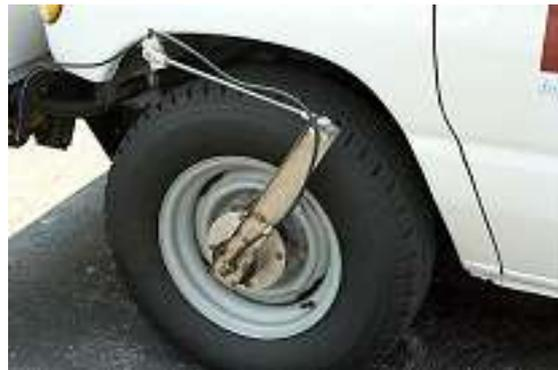
**Figure B.7 Wheel-mounted DMI (IMS, 2014)**
