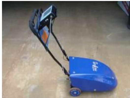
Figure C.6 ARRB Walking Profiler
