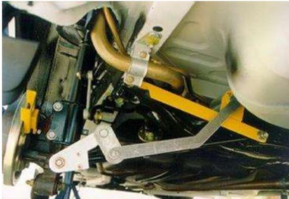
Figure C.2 Attachment of LDI suspension monitoring device to rear axle
