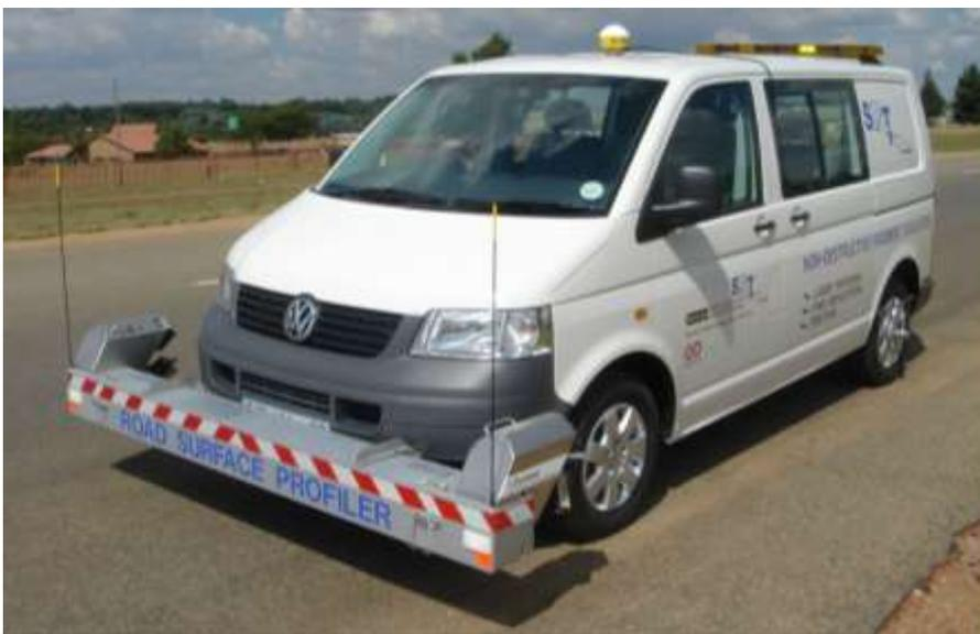
Figure C.3 Road Surface Profiler
