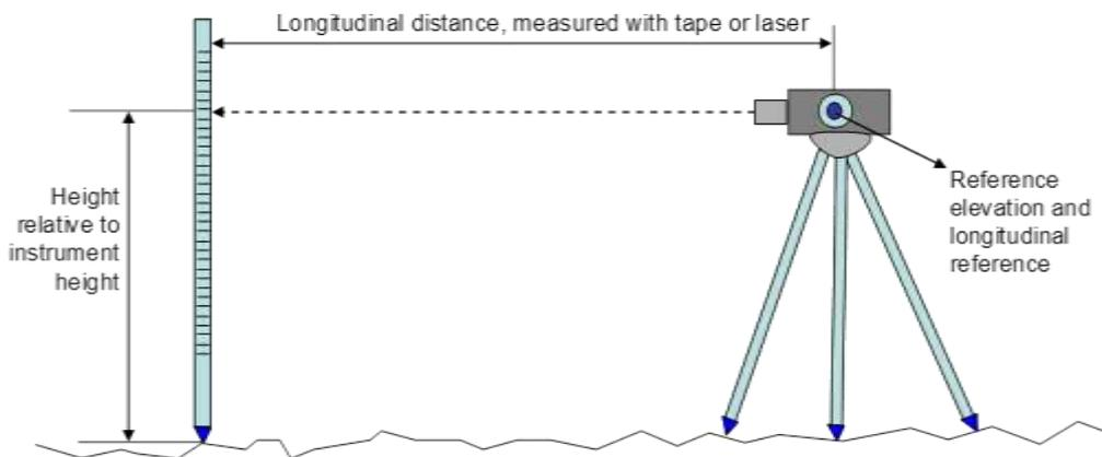
**Figure C.4 Operation of the Precision Rod and Level (after Sayers and Karamihas, 1998)**
