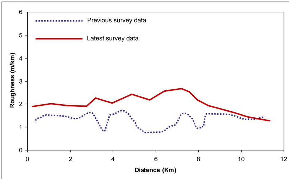
**Description:** The average IRI for the section is visibly higher and the trend in the IRI data is not the same for the two surveys.
