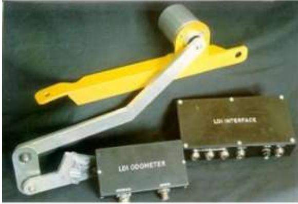
Figure C.1 Basic LDI Components, showing vertical distance measurement transducer, odometer and data capturing components
