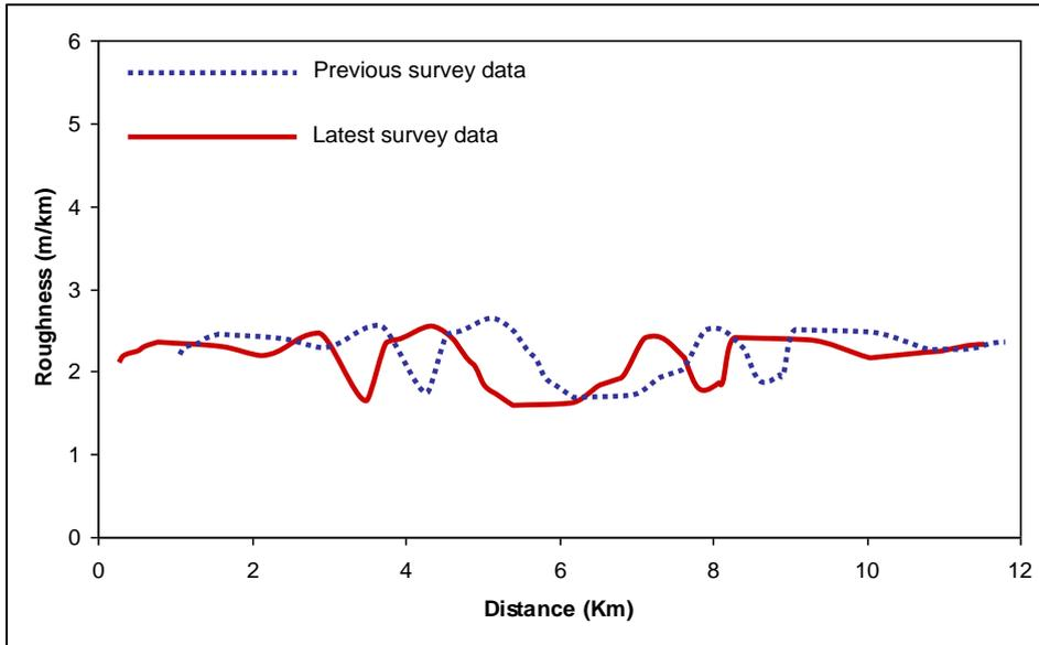
**Description:** The new data follows the same trend as that of the previous survey, and the average IRI is the same. However, the IRI at specific distance readings differs significantly.
