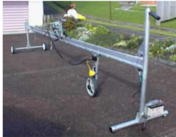
Figure D.1 Transverse Profile Beam (Bennett, 2002)
