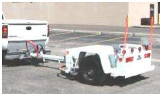
**Figure E.3 Locked Wheel Tester (Dynatest, 2008)**
