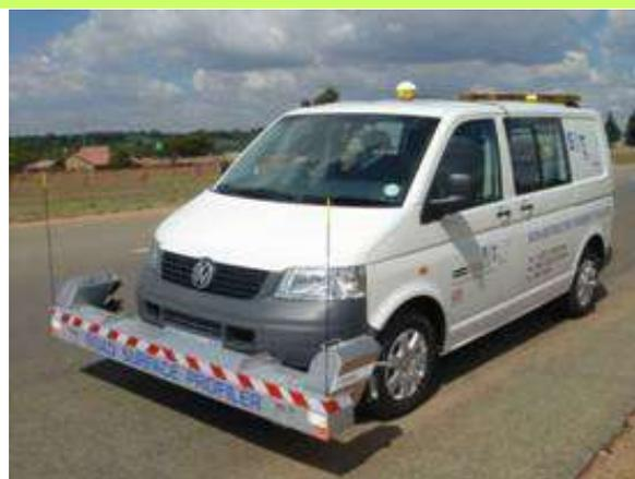
Figure E.8 High Speed Profiler (SRT, 2008)
