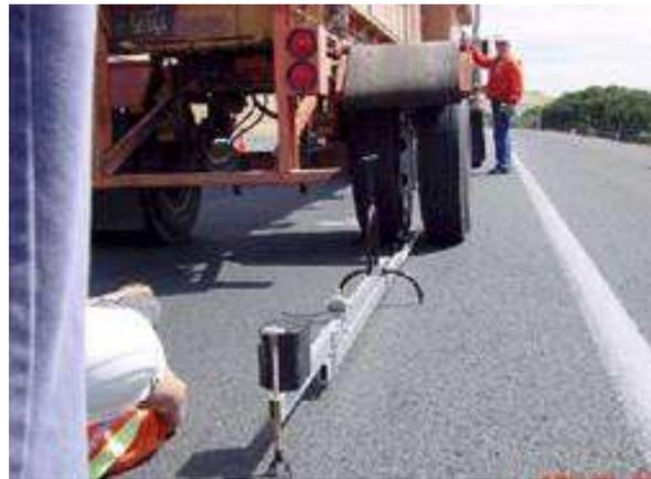
Figure F.1 Benkelman Beam (Courtesy of John Harvey)
