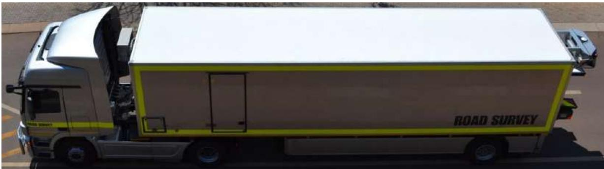
**Figure F.7 SANRAL RHINO High Speed Survey Vehicle (SANRAL, 2014)**
