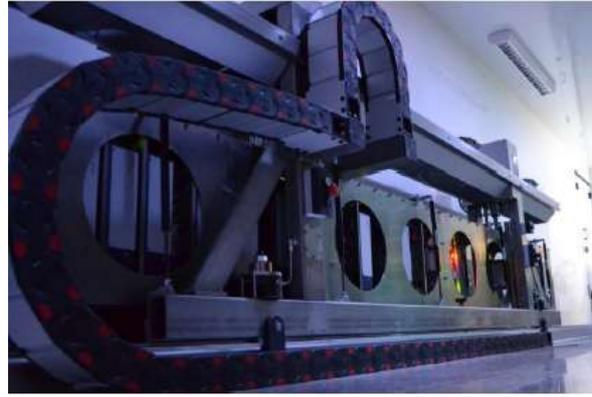
**Figure F.6 Rigid beam containing Doppler Laser sensors (SANRAL, 2014)**
