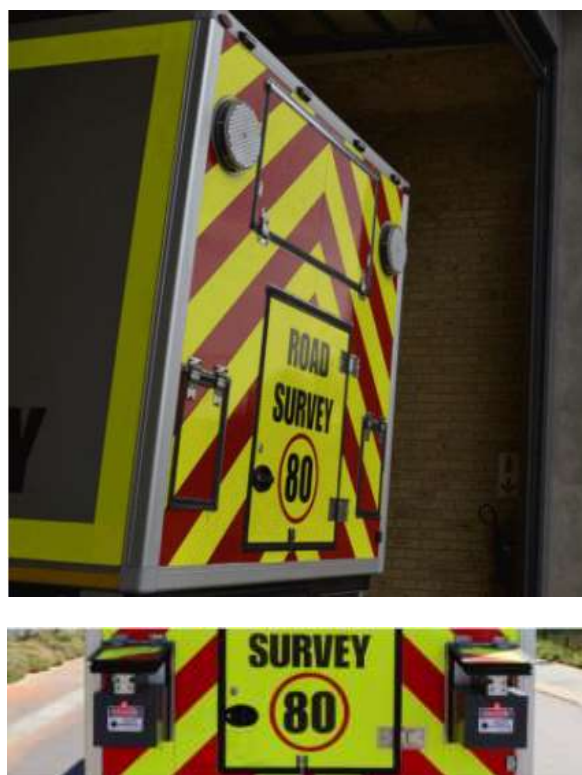
Figure G.8 SANRAL Survey Vehicle equipped with PaveVision3D Vision Ultra (SANRAL, 2014)
