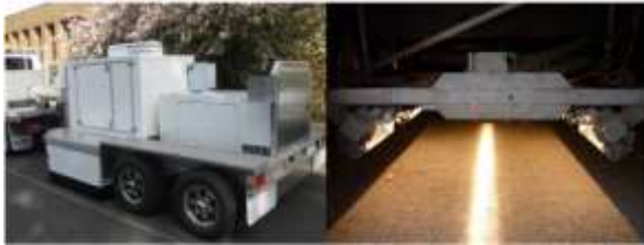
Figure G.4 RoadCrack trailer and pavement lighting (Wix and Leschinski, 2012)
