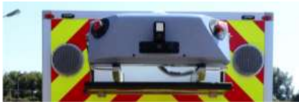
Figure G.11 SANRAL Survey Vehicle equipped with Trimble MX8 LIDAR (SANRAL, 2014)
