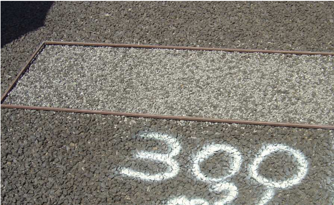
Figure F-1 Determining appropriate aggregate spread rate on site
