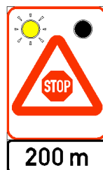
Flashing yellow warning signal SS3
