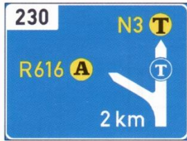
Pre-Advance Exit Direction (Class A1 Freeway)
