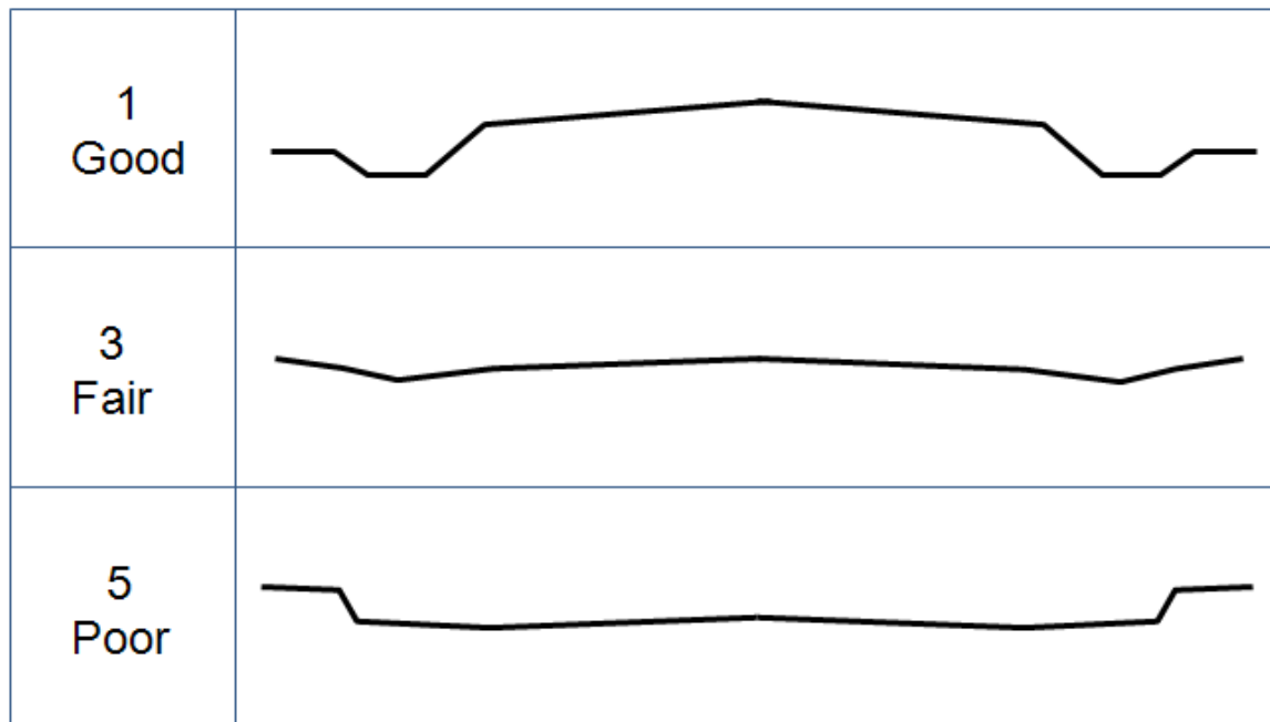
Figure 19 Guideline for rating side drainage effectiveness
